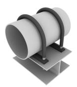
Corrosion between pipe supports and pipe at metal to metal contact points is a common problem in the process industry. TRI•GUARD™ thermoplastic bars placed under the pipe and around u-bolts, when lateral pipe restraint is required, eliminate most metal to metal contact and therefore the resultant corrosion. With TRI•GUARD™, water no longer pools on pipe support surfaces under the pipe. Water runs off due to the TRI•GUARD™ shape. TRI•GUARD™ prevents
